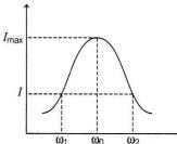
Now, as resistance is independent of frequency. So, current will same when impedance Z at two frequencies is same. At lower frequency, capacitive reactance is more but at higher frequencies, inductive reactance dominates.
